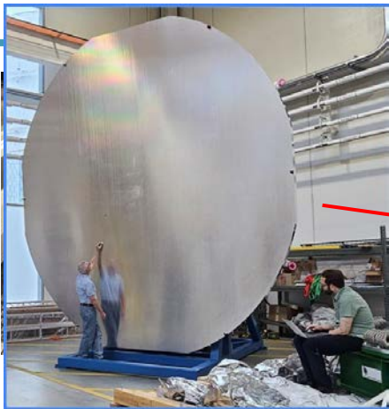
TMA Primary mirror prototype successfully fabricated and characterized
