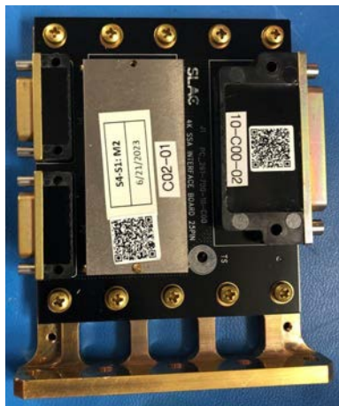
4K amplifier module with SQUID amplifiers.
