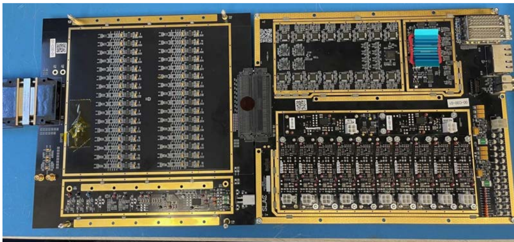
Warm Electronics row address module with FPGA board and row address front-end module
